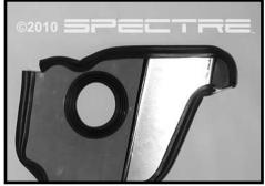
Step 8 Install the bulb seal and the 4" grommet on heat shield as shown.
