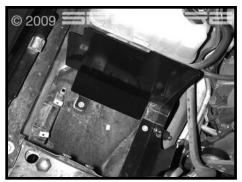
Step 11 Install the filter shield as shown, using 3 of the stock bolts removed in step 8. Fully tighten the bolts.
