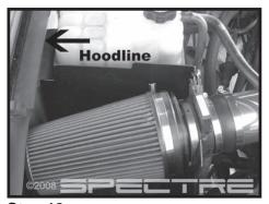
Step 18 Gently close the hood and check to make sure the intake assembly does not come in contact with the hood when closed. Make any adjustments if necessary.
