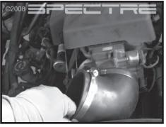
Step 10 Slide the 4" angled coupler and two 4" hose clamps over the throttle body. Do not tighten the clamps at this time.
