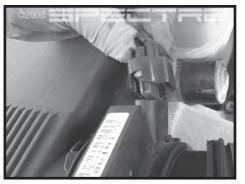
Step 4 Disconnect the MAF sensor.
