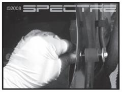
Step 9 Place the rubber vibration mount, fender washers and M6 lock nuts on the side of the housing as shown. Do not tighten the bolts at this time.
