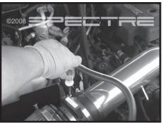
Step 17 Secure the vibration mount and tighten all the hose clamps. Do not over tighten. Reconnect the MAF sensor wiring connector.
