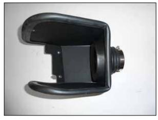
9. Install the filter adapter and coupler onto the heat shield using the provided hardware.
