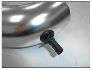
7. Using the provided grommet, install the factory Inlet air temperature sensor into the intake tube.
