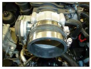
6. Install the provided coupler onto the throttle body and secure with the provided hose clamp.
