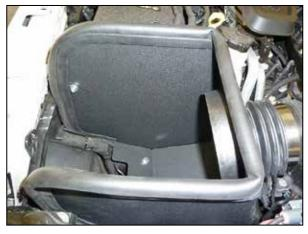
10. Install the heat shield so the mounting studs insert into the mounting grommets and secure to the rubber mounted stud with the provided hardware.
