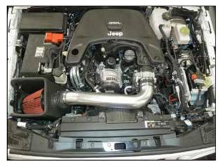
13. Make sure that all clamps and hardware are fully tightened. Reconnect the battery cable, start the vehicle and let it warm up. Shut off and inspect the installation once more for any loose clamps, wires, or hardware. Test drive & enjoy! Your installation is now complete. Periodically check all clamps and brackets.
