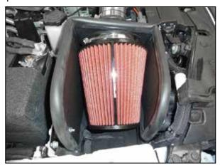
12. Install the air filter into the onto the filter adapter and secure with the provided hose clamp.
