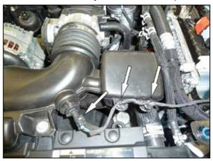
2. Disconnect the Inlet air temperature sensor electrical connection and unhook the harness from the intake plenum.
