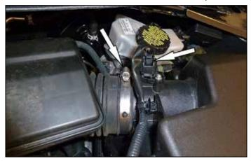
5. Disconnect MAF sensor connector by raising safety tab and push down. Release harness clips from air box. Loosen air boot hose clamp.
