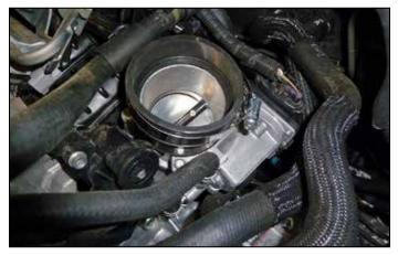
8. Install the Spectre® reducer coupler onto throttle housing and secure with provided clamp.
