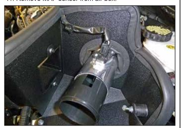
12. Push the Spectre® air intake tube through the right side of the heatshield and into coupler on throttle housing and tighten hose clamp. Install MAF sensor into intake tube with the two 4mm screws provided, then route MAF connector wiring through slot in heatshield under edge trim. Slide MAF calibration sleeve into intake tube.
