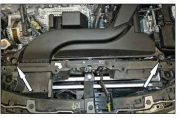
4. Remove the two bolts securing air intake duct and remove duct. This will be reinstalled in a later step.
