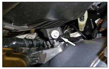
6. Remove bolt on right side of air box then remove air box from vehicle.
