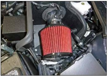
14. Place the Spectre® high flow air cleaner onto intake tube making sure calibration sleeve is located properly and tighten clamp.
