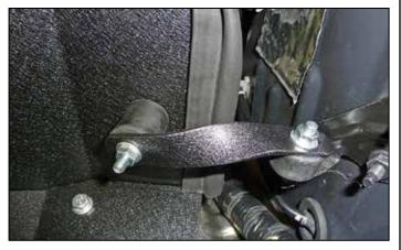
10. Install twist bracket and rubber mounts with hardware provided as shown.
