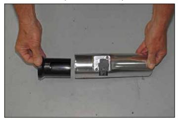
9. Remove the mass air sensor from the factory intake system and then install it into the SPECTRE<sup>®</sup> intake tube. Install the maf sleeve into the intake tube as shown, the sleeve should slide all the way in until the lip contacts the end of the tube.
