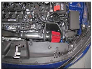
12. Reconnect the maf sensor electrical connection.
