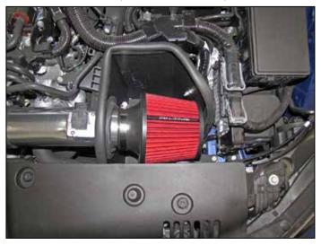
11. Install the SPECTRE<sup>®</sup> air filter onto the intake tube and secure with the provided hose clamp.
