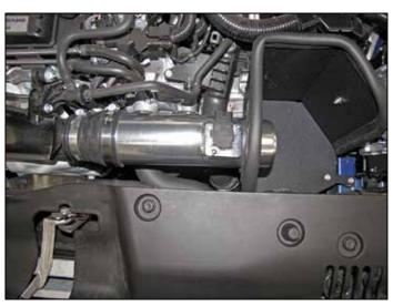
10. Install the SPECTRE<sup>®</sup> intake tube into the heat shield and then into the coupler hose, adjust for best fit and then secure with the provided hose clamp.
