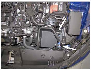
6. Install the heat shield assembly into the vehicle and secure with the provided hardware where shown.
