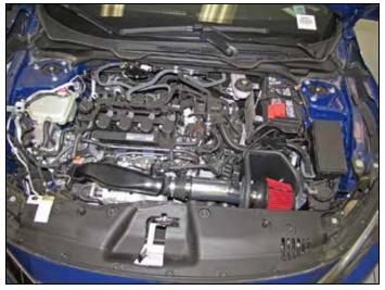
**13. Double check your work!** Make sure there is no foreign material in the intake path. Make sure all clamps, hoses, bolts, and screws are tight. Double check the hood clearance! **Reconnect the negative battery cable!**
