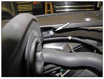
7. Secure the front of the heat shield to the core support with the provided hardware as shown.
