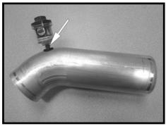
Step 13 Install the provided grommet into the Spectre intake tube then, install the filter minder into the grommet.
