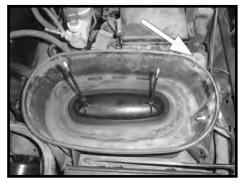
Step 5 Loosen the nut that secures the lower air cleaner assembly as shown.
