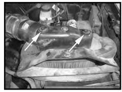
Step 3 Loosen the screws that secure the air cleaner top as shown.
