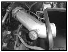
Step 17 Install the Spectre intake tube into the hole in the heat shield then, into the flex coupler at the turbo inlet tube. Secure with the provided hose clamps.
