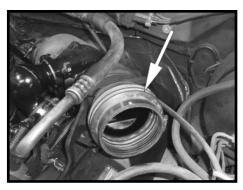
Step 10 Install the provided 4" flex coupler onto the turbo inlet tube using the provided hose clamps.
