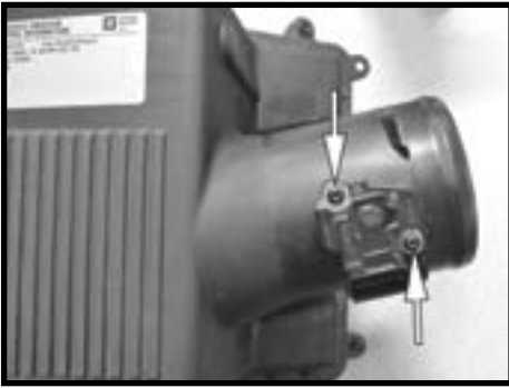
Step 8 Remove the MAFS sensor from the factory air box.
