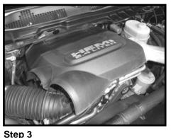
Remove the engine cover by lifting up to release the rubber mounts securing it to the motor. Then pull it forward and remove the cover from the vehicle.
