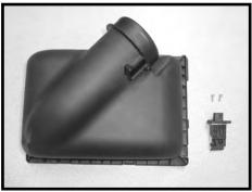
Step 6 Remove the Mass Air Meter from the stock air box.
