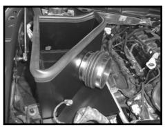
Step 9 Install the heat shield, using the 4 factory clips from the airbox, clip heat shield into position.
