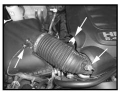
Step 2 Disconnect the IAT sensor connector, the Mass air meter connector and the PCV quick disconnect hose.
