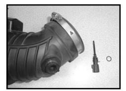
Step 5 Remove the IAT sensor from the stock intake tube. Lift up on the locking tab and rotate the sensor counter clockwise and pull it out. Then remove the o-ring from the sensor.
