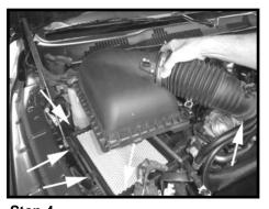
Step 4 Loosen the clamp on the intake tube at the throttle body. Unclip the four hold down clips on the air filter lid. Remove the intake tube and airbox lid assembly from the vehicle. Remove the stock air filter.
