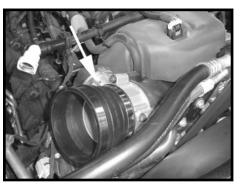
Step 10 Install the provided reducer coupler onto the throttle body as shown.
