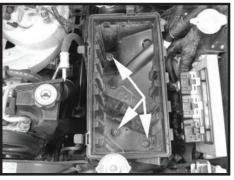
Step 4 Remove the two bolts and one nut in the bottom of the air box and remove air box from vehicle. The nut will be reused in a later step.
