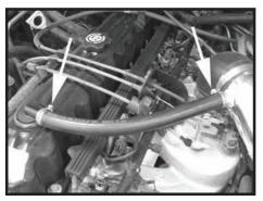
Step 11 Install the supplied crank case vent hose and fasten it securely in place.
