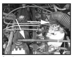
Step 2 Loosen the clamp at the throttle body. Remove the crank case vent hose from the fitting on the valve cover.
