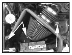
Step 8 Install the heat shield into the vehicle as shown by reusing the hardware from Step 4 and Step 7.
