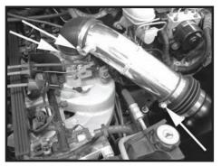
Step 10 <u>Install the intake tube</u> into the flex coupler and then install the 90° coupler to the intake tube and then position it onto the throttle body as shown. Once in desired position fasten it securely in place.
