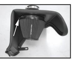
Step 6 Install the filter and securely fasten to the velocity stack adaptor.
