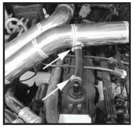
Step 19 Install the supplied crank case vent hose and fasten it securely in place.
