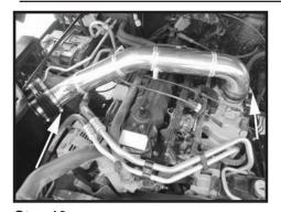
Step 12 Install the intake tube and once in desired position fasten it securely in place. If the vehicle has an IAT sensor, reconnect the sensor at this time.
