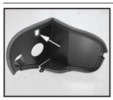
Step 7 Install the 1/16" edge in area shown with the arrow. This may require trimming to the correct length. Install the edge trim around the edge of the heat shield. This may require trimming to the correct length.
