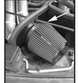
Step 20 <u>Install the filter</u> and securely fasten to the velocity stack adaptor.
