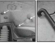
Step 3 Remove the air filter and locate the three mounting nuts on the inside of the fender well. Remove the nuts and remove the air box base from the engine compartment. The pictured components will now be out of the engine compartment.
