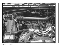
Step 2 Loosen clamp at throttle body. Remove the crank case vent hose from 90° fitting. If present, disconnect the IAT electrical connector. Unclip air box cover. Lift entire assembly from engine.
