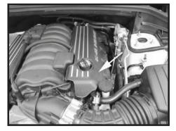
Step 2 Remove the engine cover.
