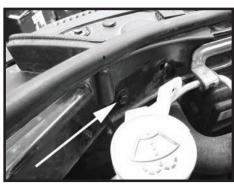
Step 12 Remove the bolt on the core support. This will be reused in the next step.
