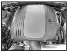
Step 16 Install top engine cover. Position the breather hose so it does not rub on cover.
