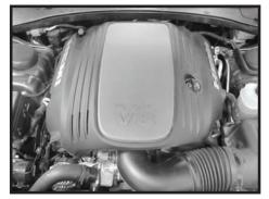
Step 2 Remove the engine cover.
