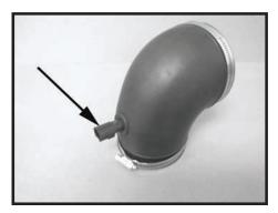
Step 7 Install the supplied grommet into the 90°coupler then install the IAT sensor into the grommet. Install the hose clamps on the coupler.
