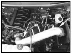
Step 10 Install the Spectre Performance intake tube into the flex coupler on the heat shield then into the coupler on the throttle body. Fasten securely in place.
