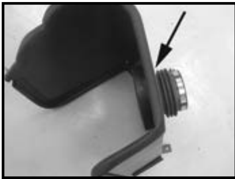
Step 11 Place the velocity stack adapter in the heat shield and install the supplied flex coupler making sure the coupler is pushed completely against the heat shield. Once the adapter and coupler are tight against the heat shield, tighten the clamp. Install a second clamp but do not tighten at this time.
