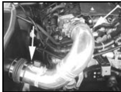
Step 15 Install the intake tube as shown and once in position tighten clamps.
