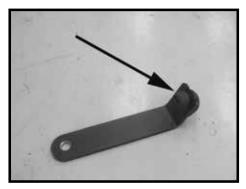
Step 6 Install the grommet removed on Step 5 into the supplied bracket.
