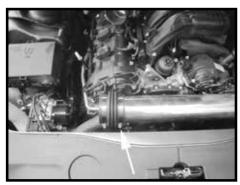
Step 15 Install the flex coupler onto the end of the tube and fasten it securely, leave the other clamp loose at this time.
