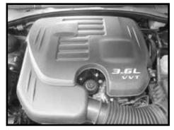
Step 2 Remove the engine cover.
