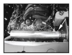
Step 14 Install the intake tube as shown making sure the small vent tube closest to the heat shield.
