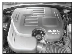
Step 2 Remove the engine cover.
