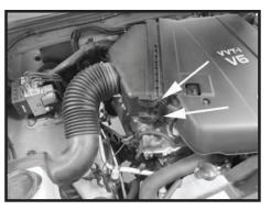
Step 3 Unclip the air box lid from the vehicle and remove the lid assembly from the vehicle.
