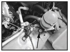
Step 4 Remove the screw that secures the power steering reservoir to the vehicle. The screw will be reused in Step 9.
