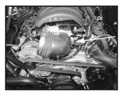
Step 15 Install the 90° boot on throttle body with the short side on the throttle body and clamp on the throttle body side to secure the boot in place. Install a second clamp but do not tighten at this time.
