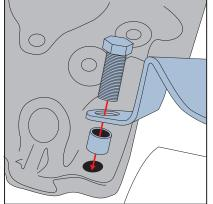
Once the belt is installed over the alternator pulley install but do not tighten upper alternator bolt (included with alternator). Tighten all bracket bolts, slide alternator to the location where the correct belt tension is achieved (refer to manufacturers specifications) and tighten the final alternator bolt in place.
