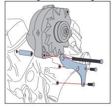
Install short (1") bolt through upper bracket into water pump, if needed use the short (.5") spacer but do not tighten. Install the medium length bolt (2.5") through the upper bracket, through the medium spacer (1") and into the manifold bolt hole but do not tighten completely.
