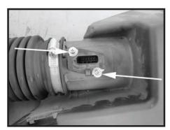
Step 11 Remove the two screws that secure the MAFS to the factory air box and remove the MAFS.
