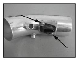
Step 12 Install the MAFS into the Spectre Performance intake tube and secure with the supplied screws.
