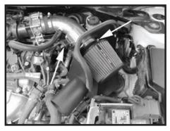
Step 17 Reconnect the MAFS electrical sensor. Install the filter and fully tighten clamp.
