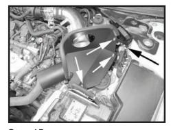
Install the heat shield into the vehicle and position it so the mounting holes line up with the rubber mounted studs installed in step 8 and the intake tube is in the center of the opening. Secure the heat shield with the supplied lock nuts and washers. Secure the heat shield bracket on the inner fender with the hardware provided. Tighten the bolt securing the other end of the heat shield bracket.
