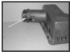
Step 6 Remove the MAFS from the factory intake tube
