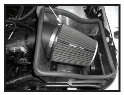
Step 14 Install the supplied air filter and clamp and tighten the clamp that secures the air filter. If needed, rotate the air filter/velocity stack adapter assembly for the maximum clearance as shown.
