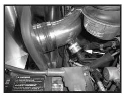
Step 14 Reinstall the filter minder into the tube.
