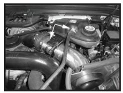
Step 13 Install the intake tube. Reconnect the MAFS and the radiator overflow line.
