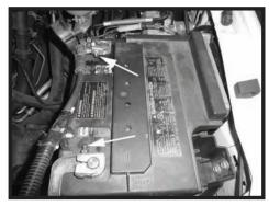
Step 10 Loosen the battery terminals and remove them from the battery. Unclip the factory battery cover and lift up  $\frac{1}{2}$ " this will allow the new heat shield to fit in place.
