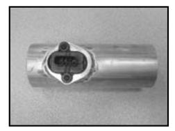
Step 9 Install mass air flow sensor into the Spectre Intake and secure with provided hardware.
