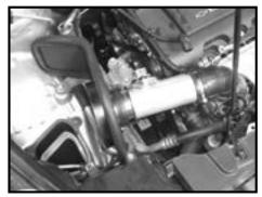
Step 13 Install the intake assembly into the factory intake elbow and align the heat shield with the rubber mounted studs installed into the mounting bracket. Align the intake for correct fit and secure with provided hardware and factory hose clamp.
