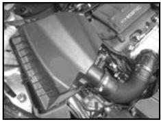
Step 4 Remove airbox assembly from vehicle by lifting up and releasing from grommets.
