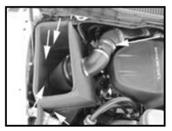
Step 8 Install the heat shield making sure that the slots on the heat shield are inserted into the lower factory air box tabs, and the MAFS is installed into the factory flex hose. With the heat shield located in the tabs, and MAFS in place, use the 4 factory clips from the air box, clip heat shield into position and securely fasten the MAFS in place.
