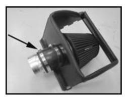
Step 6 Install the intake tube into the angled coupler and fasten securely in place.
