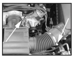
Step 4 Loosen the clamp at the throttle body and at the Mass Air Flow Sensor (MAFS). Remove the factory intake plenum from the vehicle.
