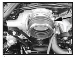
Step 17 Install the flex coupler on throttle body and clamp on the throttle body side to secure the boot in do not tighten at this time.
