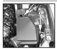
Step 7 Remove the two nuts that secure the factory air box in place. Once removed, lift the air box out of the vehicle including the factory scoop that is connected to the air box.
