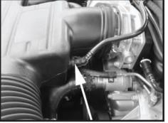
Step 3 Disconnect the breather hose that is positioned just to the right of the throttle body by squeezing the hose end and removing the hose from the air box.
