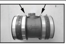
Step 13 Install the couplers on the end of the MAFS and fasten them securely in place. Install a second clamp on each coupler but do not tighten at this time.
