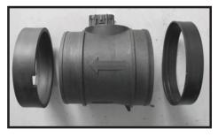
Step 12 Install the thick rubber spacer on end of the MAFS that the arrow is pointing too. Install the thin rubber spacer on the opposite end of the MAFS.
