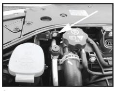
Step 10 Remove the mounting screw for the washer reservoir filler neck.
