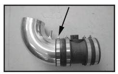
Step 14 Install the large intake tube with the MAFS pointing towards the intake tube.
