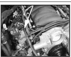
Step 8 Connect the supplied hose to the breather tube on the motor.
