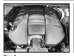
Step 2 Remove the oil cap to allow you to remove the plastic engine cover. Remove the engine top cover (if equipped) and reinstall the oil cap to ensure that nothing falls into the engine while you are working.
