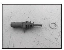
Step 11 Remove the factory O-ring from the IAT sensor.
