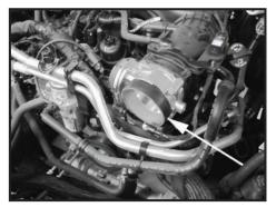
Step 6 Install the throttle body adapter ring onto the throttle body.
