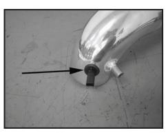
Step 12 Install the grommet into the tube. Reinstall the factory IAT sensor.
