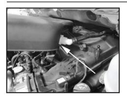
Step 5 Unclip the PCV hose from the plenum and remove the intake plenum and air box lid assembly from the vehicle.
