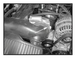
Step 3 Loosen the clamp at the throttle body.
