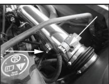
Step 18 Reconnect the MAFS wiring harness and the pressure sensor connector.
