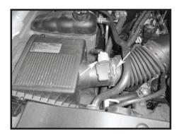
Step 4 Loosen the clamp at the Mass Air Flow Sensor (MAFS). Disconnect the MAFS electrical connector.
