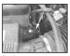
Step 5 Disconnect the pressure sensor connector.
