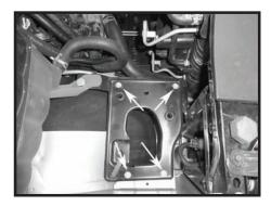
Step 9 Remove the air box mounting plate. Two of these bolts will be re installed with the new heat shield.
