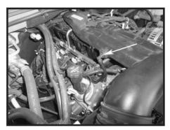
Step 6 Pull firmly and disconnect the breather hose from the stock intake resonator. Remove the factory intake tube.
