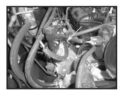
Step 16 Connect the supplied hose to the breather tube on the motor.
