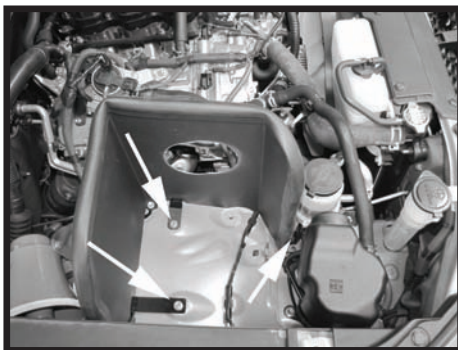
Step 14 Install the heat shield into the truck as shown with the supplied hardware and the bolt removed in Step 13.
