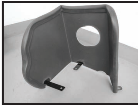
Step 12 Install the rubber bulb seal on the heat shield. This may require trimming to the correct length.
