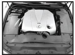
Install the engine cover. Make sure that all clamps and hardware are fully tightened. Reconnect the battery cable, start the vehicle and let it warm up. Shut off and inspect the installation once more for any loose clamps, wires, or hardware. Test drive & enjoy! Your installation is now complete. Periodically check all clamps and brackets.
