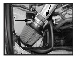
Step 20 Install the supplied air filter and secure it with the supplied clamp. Reconnect the electrical connector to the MAFS.
