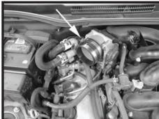
Step 16 Install the coupler on the throttle body and fasten securely. Install the second clamp but do not tighten at this time.
