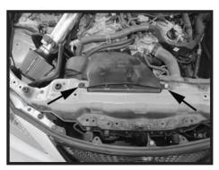
Step 21 Install the factory fresh air duct with the factory bolt and clip that was removed in step 4.
