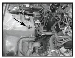
Step 6 Install the supplied rubber mount onto the closest hole on the inner fender panel.
