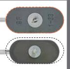
Larger float has better buoyancy which increases fuel gauge accuracy
