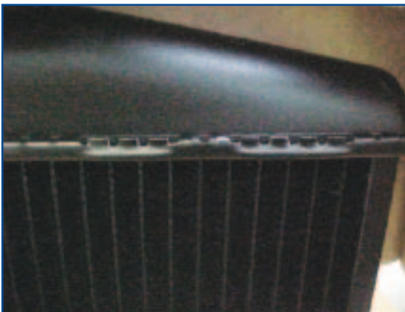
Example of poor crimping
