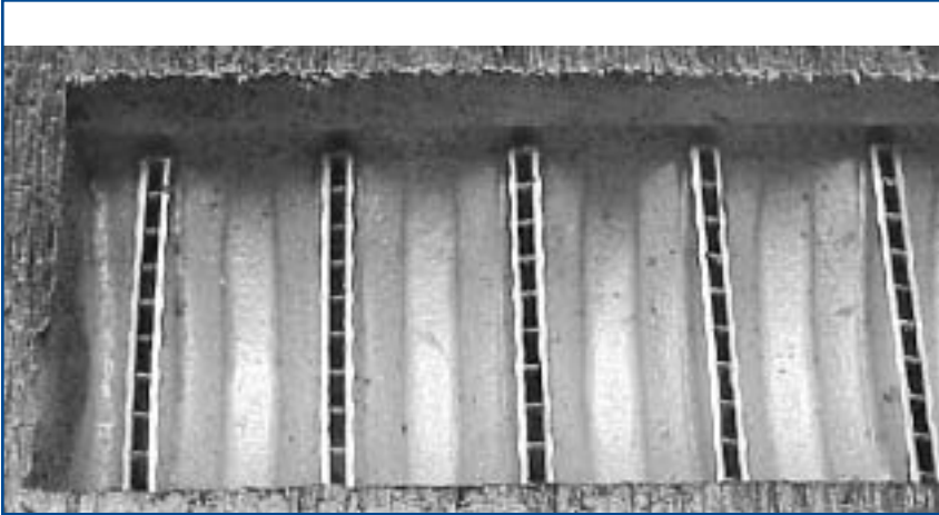
Cutaway View of Parallel Flow Condenser Tubes
