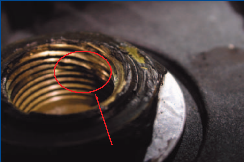
Stripped oil cooler threads
