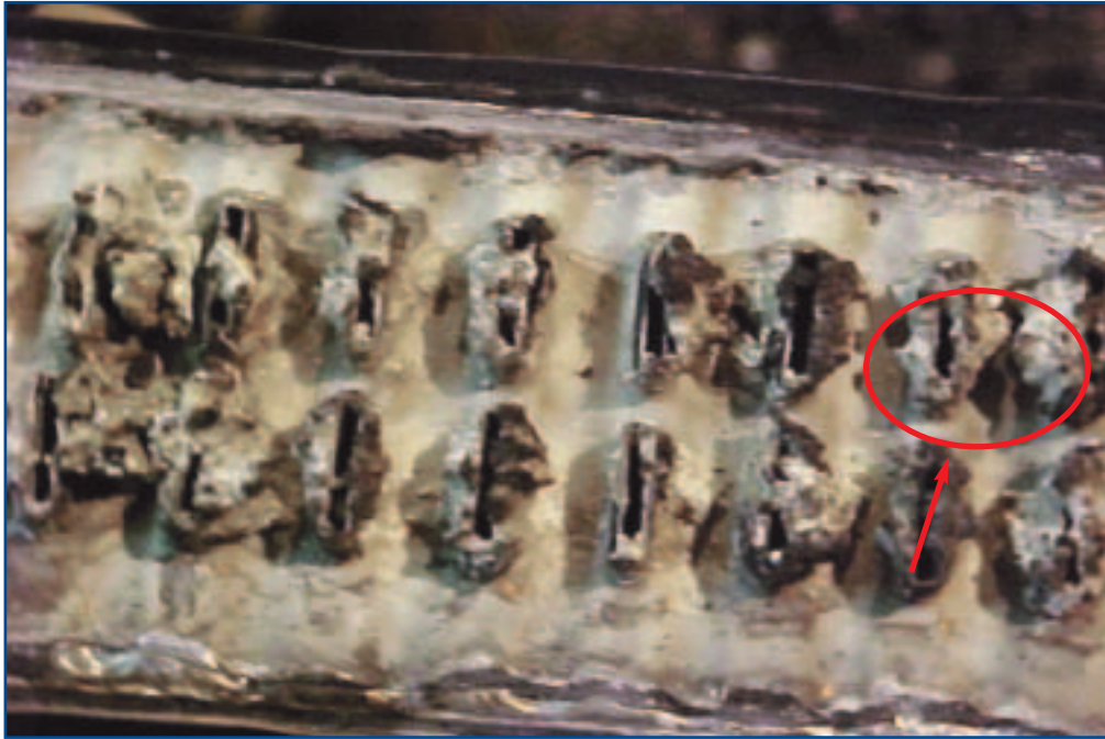
Solder bloom resulting of contaminated coolant, which creates restricted flow within the radiator
