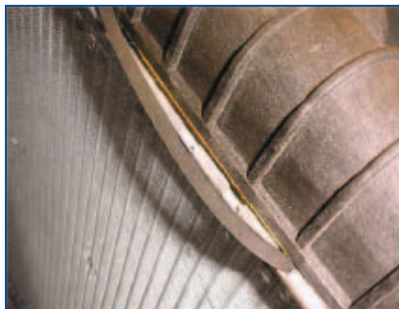
Blown Seam on a Plastic Aluminum Radiator
