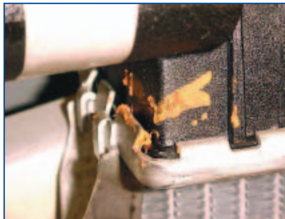
Example of a bad end crimp
