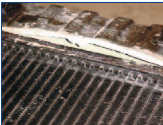
Blown Tank Seam
