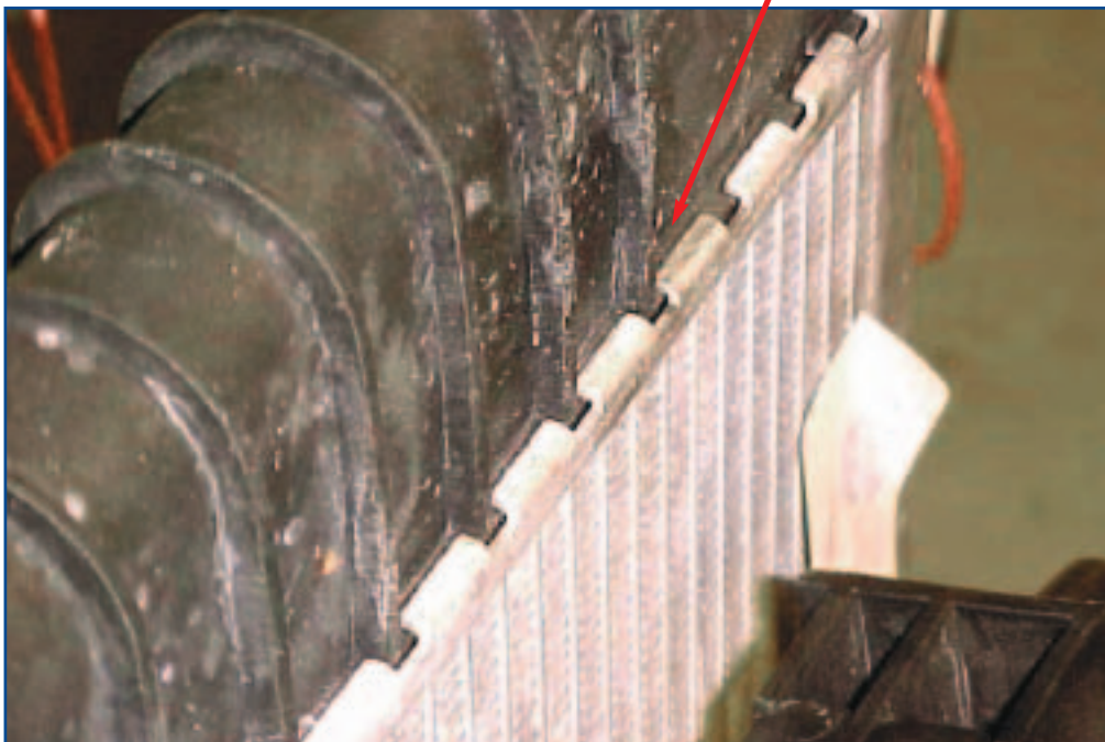
Tank Seam Leak due to a bad crimp or faulty gasket
