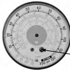
CHECK YOUR LOW SIDE GAUGE WHEN EMPTY. IF IT'S NOT ON ZERO, RECALIBRATE IT.
