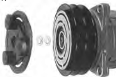
ADJUST AIR GAP BY CHANGING SHIMS
