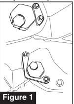
unload the suspension and start with the cam bolt positioned for the most positive camber.
