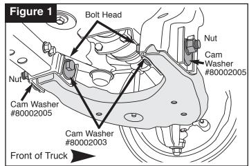
Adjust toe and road test vehicle.
