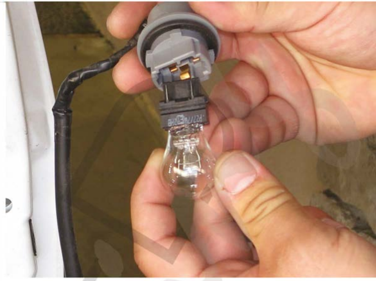
6. Remove the brake light bulb
