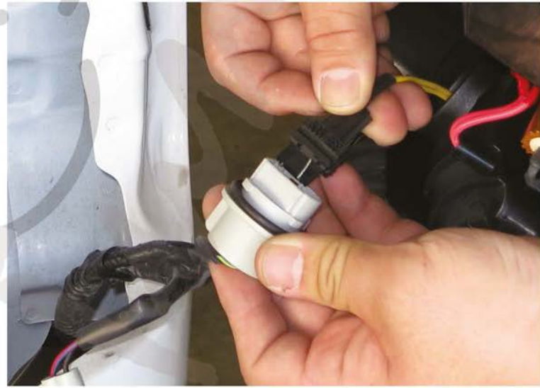
8. Connect the taillight harness to LED taillight
