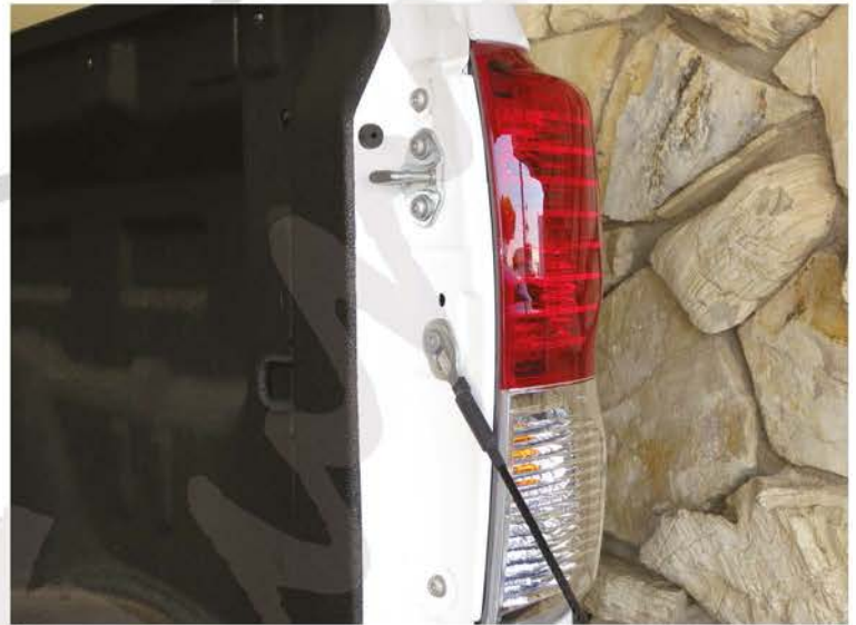
2. 2 T30 bolts location
