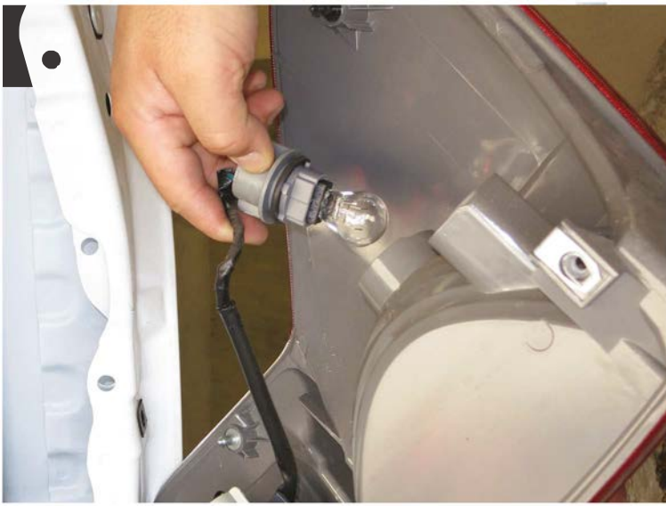
5. Remove the light sockets
