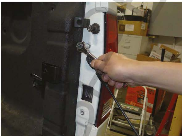
3. Remove the (2) 10mm bolts
