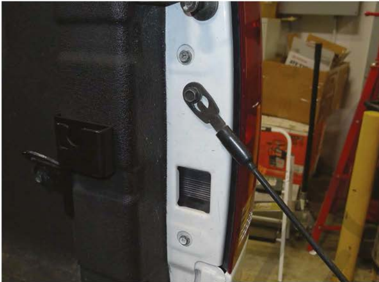
1. (2) 10mm bolts location
