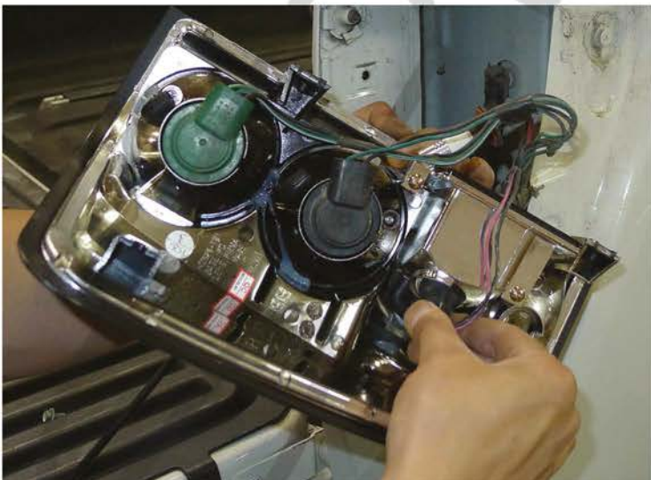
15. Install the taillight socket into the LED taillight
