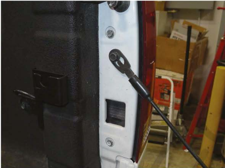
1. (2) 10mm bolts location
