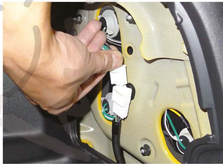
8. Connect the taillight harness
