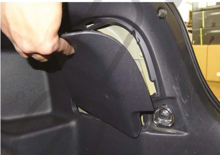
9. Replace the access hole cover.
