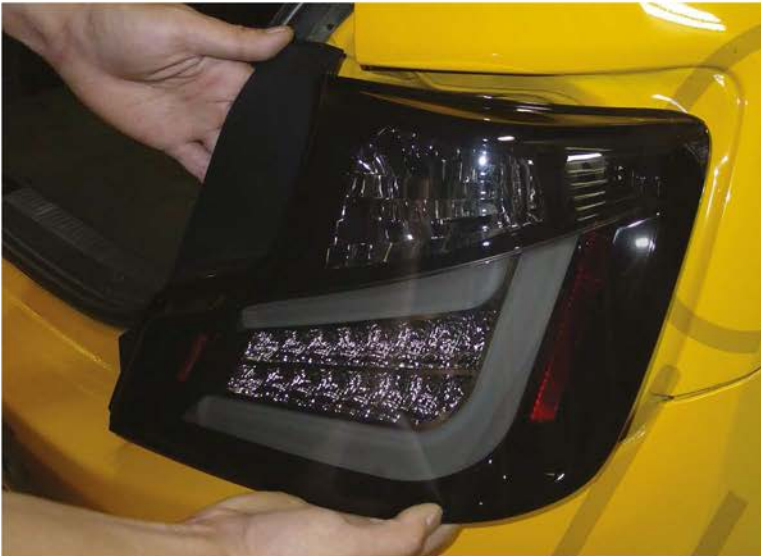
7. Place the LED taillight in the stock position
