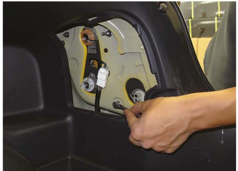
4. Remove the (3) 10mm nuts
