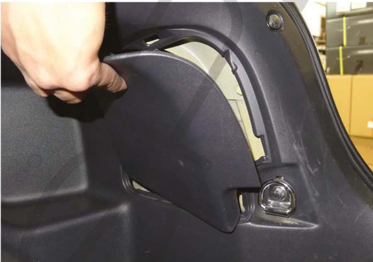
9. Replace the access hole cover.
