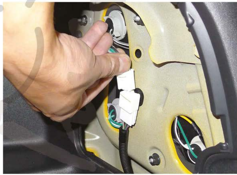
8. Connect the taillight harness
