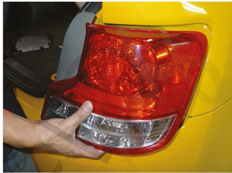
6 Remove the factory taillight
