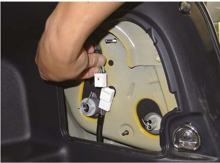
5. Disconnect the taillight harness
