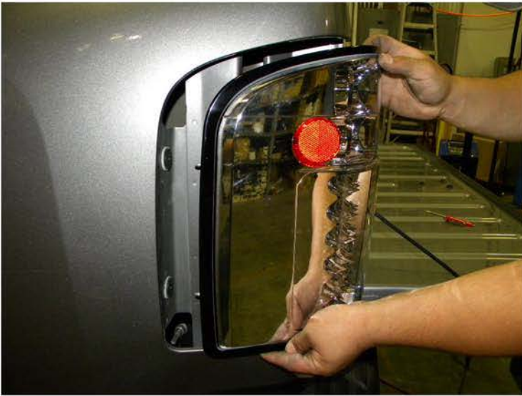
11. Place the LED tail light onto the vehicle
