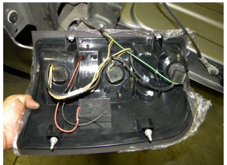
10. Place the socket into the LED tail light assembly
