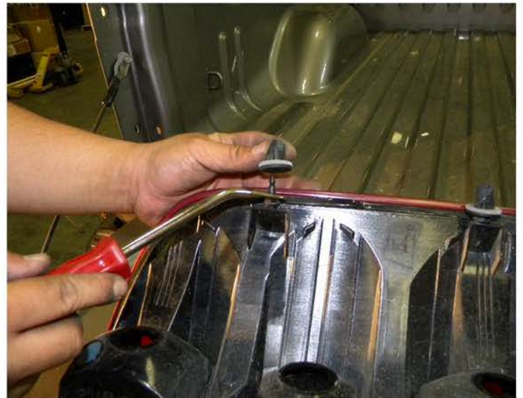
4. Remove the (2) plastic holders from the tail light
