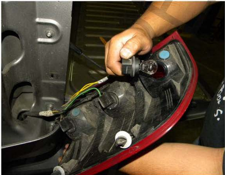
3. Remove the harness and bulbs from the tail light
