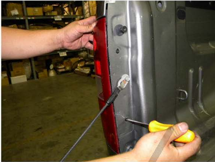
1. Remove the (2) Phillips head screws
