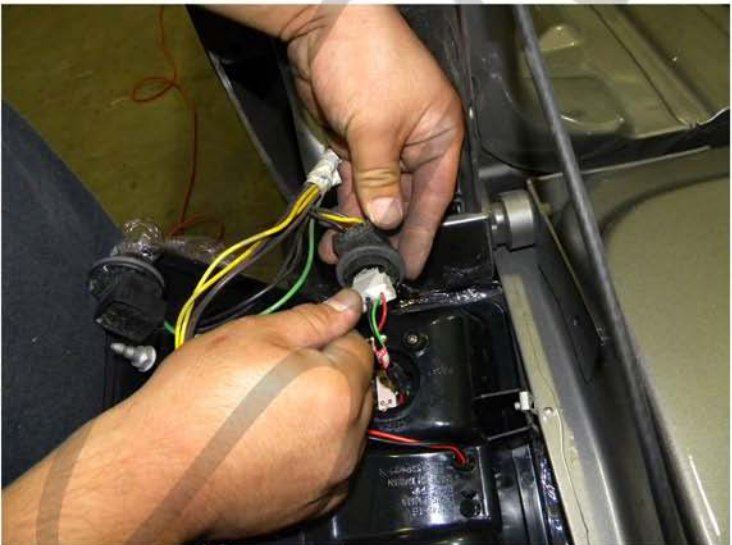
8. Connect the LED tail light connector into the tail light harness
