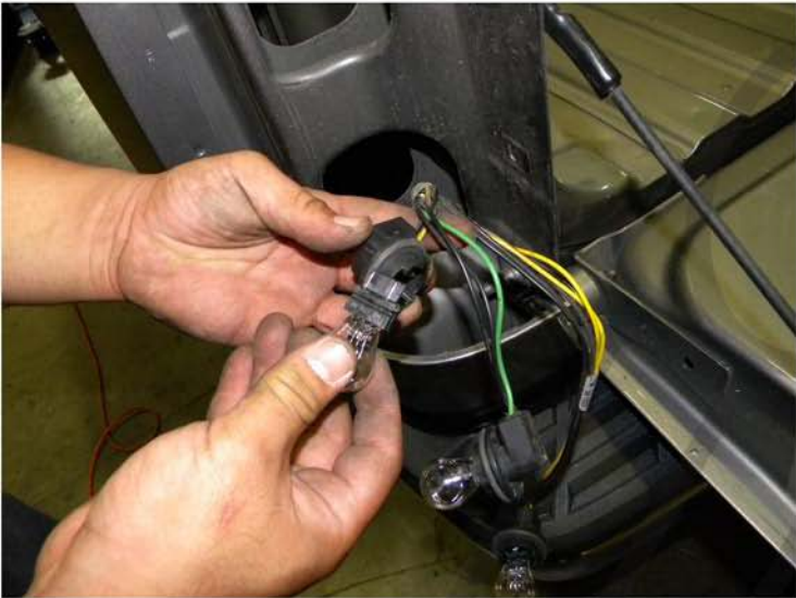
7. Remove (2) light bulbs from harness, brake, and signal lights
