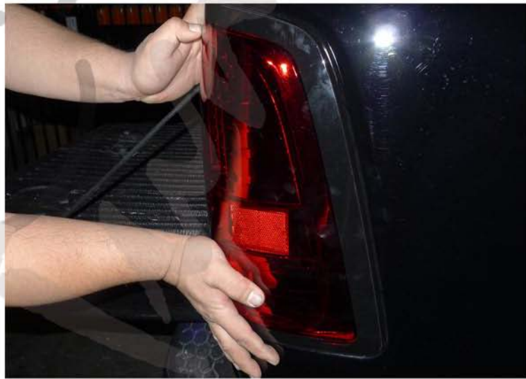
8. Place the LED taillight in the stock location
