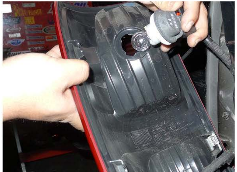
4. Remove the taillight sockets
