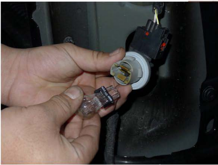
5. Remove thr brake light bulb
