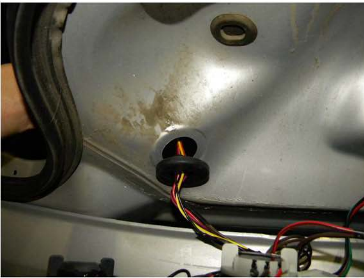
11. Run the tail light harness through the body work please see the "L.E.D. tail lights installation instruction" If your tail lights don't have L.E.D. You can skip the installation instruction.
