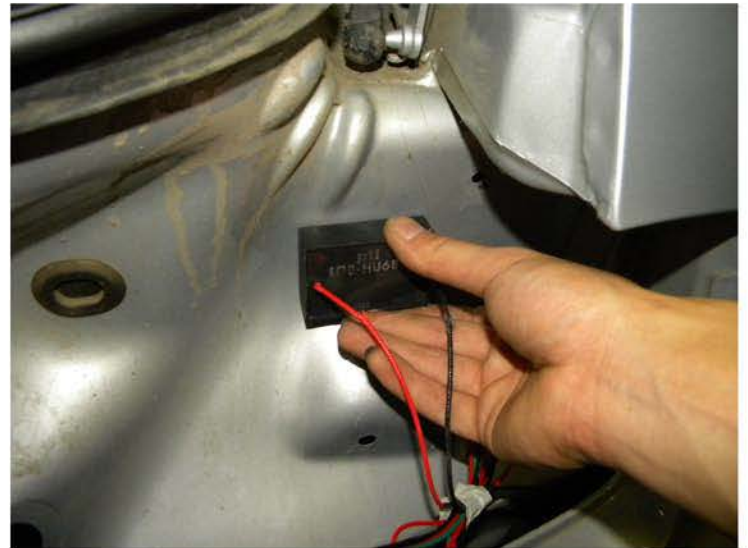
10. Secure the LED resistor block and harness to the body with double sided foam tape
