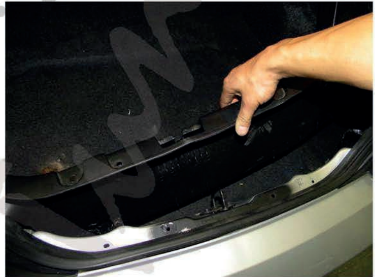
14. Replace Plastic trunk moulding
