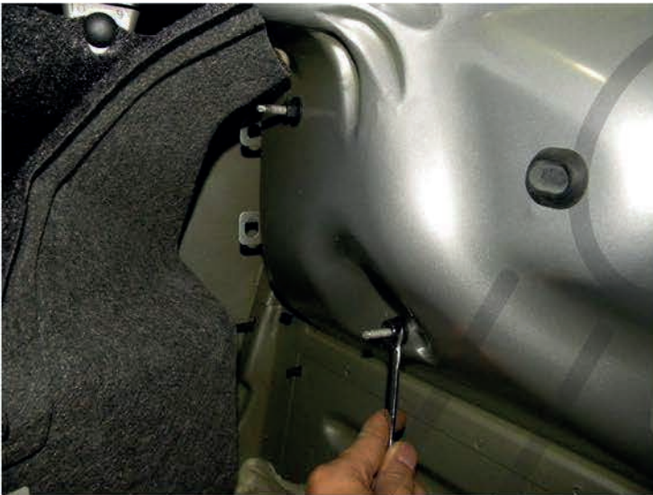
13. Tighten (3) 10mm bolts
