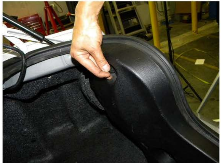
4. Remove the (6) plastic clips
