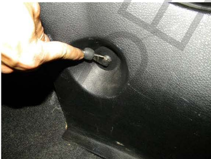
3. Remove the (6) plastic clips
