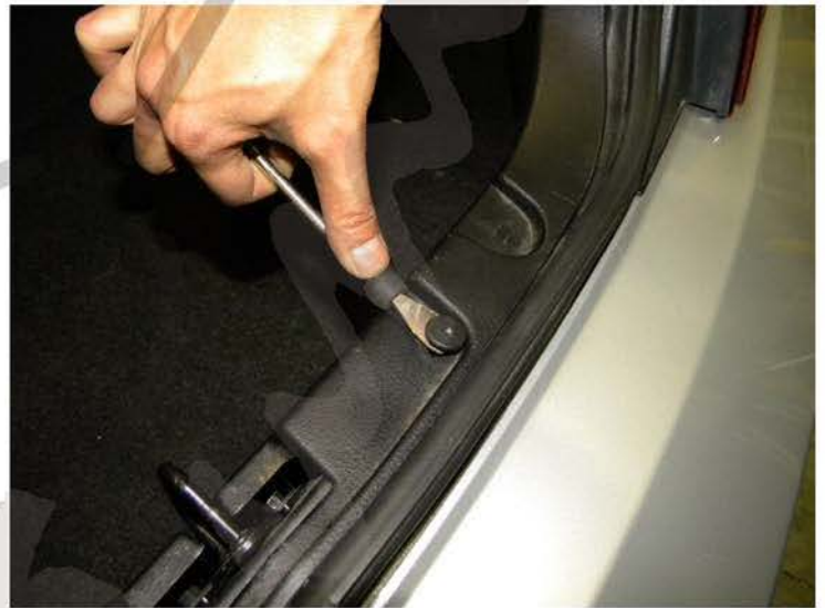
2. Remove the (6) plastic clips
