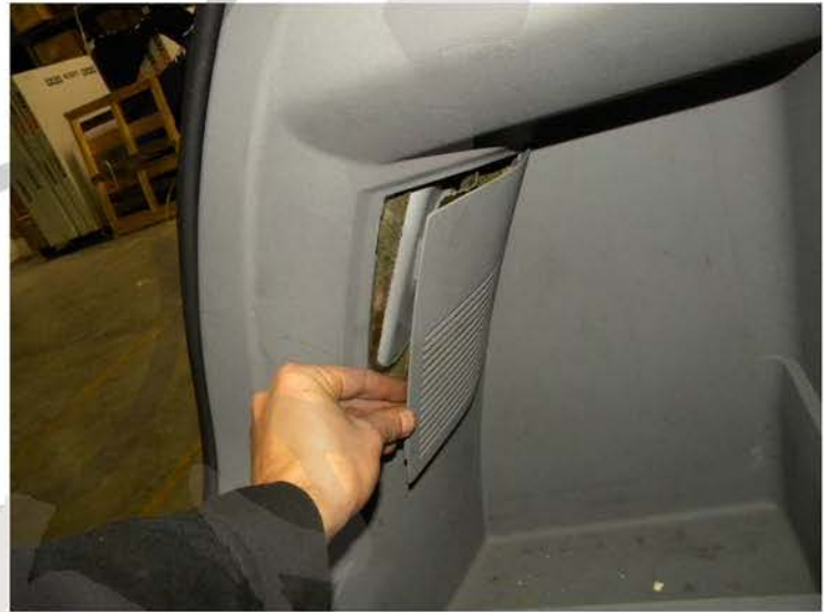
2. Remove the cover from inside of the trunk
