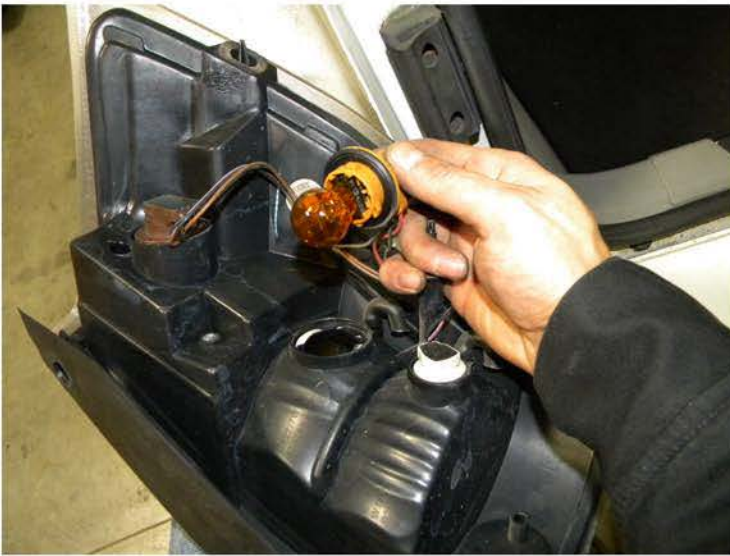
5. For Altezza Taillight, remove the the wire harness from the OEM taillight then install the wire harness to the new Taillight Please see the L.E.D.Tail Light wire installation instruction
