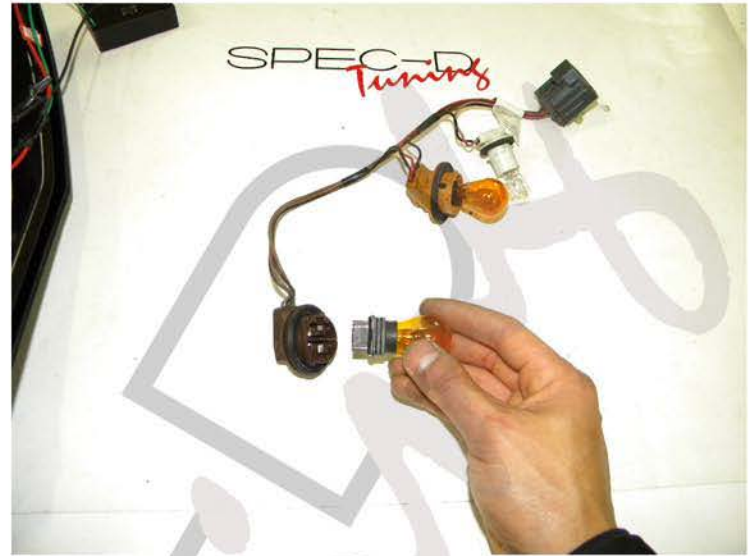
6. For LED Taillight, you need to remove the brake light light bulb to install the wire harness to the new LED taillight
