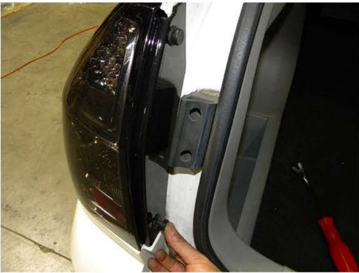
11. Install two clips please repeat the picture order from 1 to 11 for the opposite side
