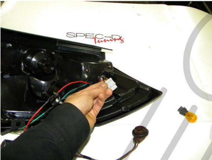
7. Plug the harness into the sockets
