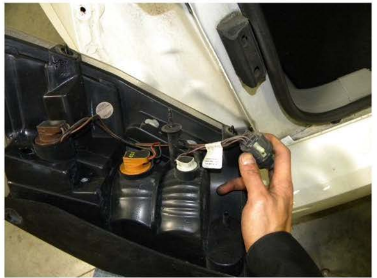
4. Disconnect the taillight wire harness then remove the taillight
